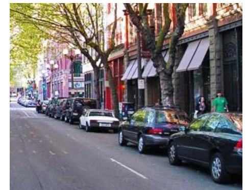
On-street parking may act as a buffer by separating pedestrians from moving vehicles on the road.
